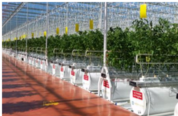
Treated air is pumped through sleeves that are under the plants, or is released above the plants.
