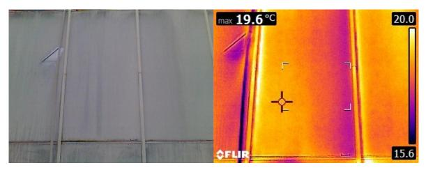
In the thermal image, there is a small red cross near the centre of the image, which shows where the camera is measuring the temperature. So, the 19.6°C refers to the location of the red cross, which in this image is on the surface of the glass.
