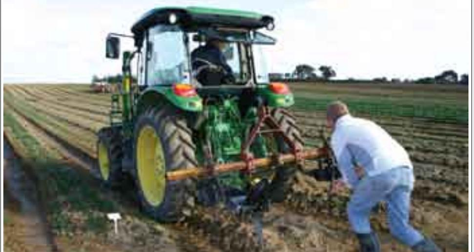
**Horowhenua grower John Clarke tests the furrow diking equipment at his Woodhaven Gardens operation (top). The outcome is a series of small soil dams in the wheel track that slow water movement (bottom).**
