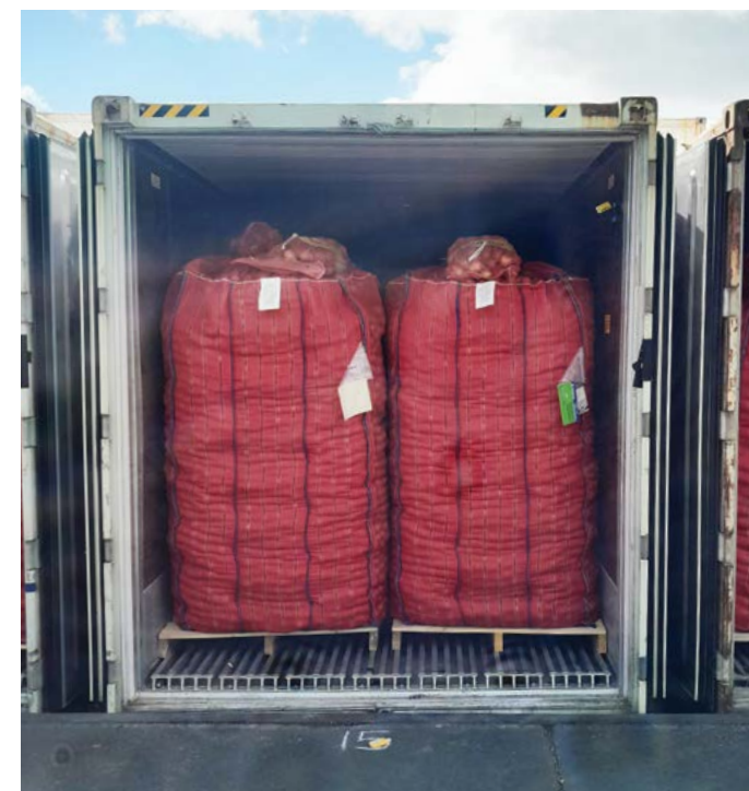
Effective airflow to regulate temperature requires even loading patterns that avoid product being loaded against the walls of the container
