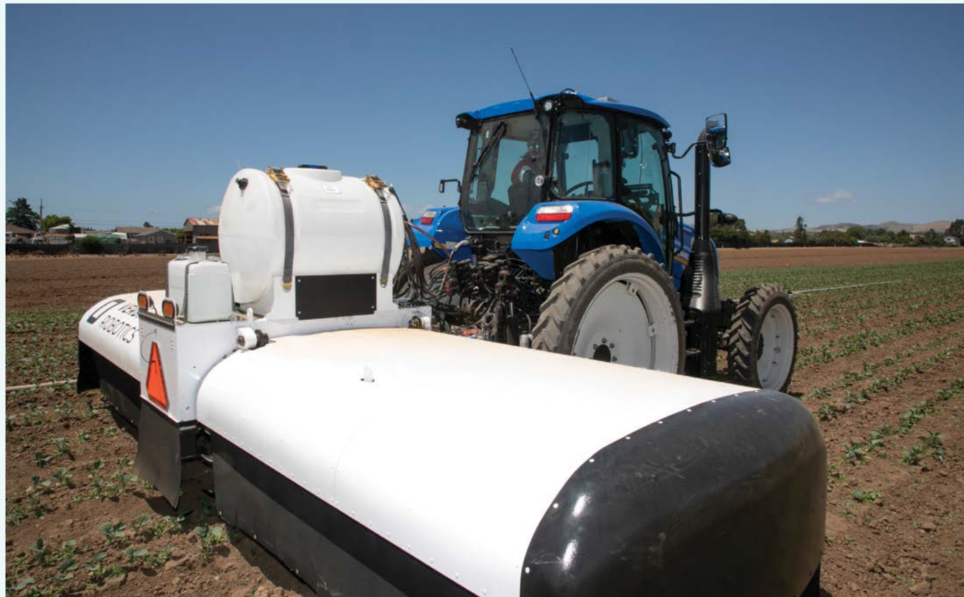
Verdat Robotics from the United States manufactures a spot sprayer that identifies weeds and avoids blanket spraying. Photo courtesy of Callaghan Innovation
