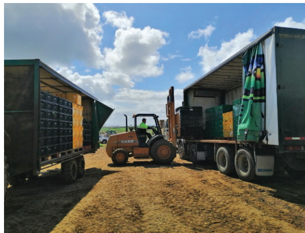
Figure 3.4: Use of trans-shipping principles to keep harvest machinery on the blocks and trucks on loading pads.
