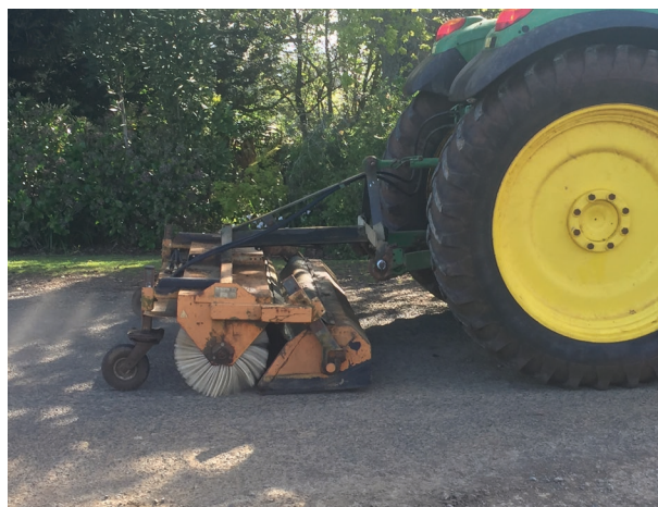
Figure 3.6: Road sweeping device mounted on a tractor.
