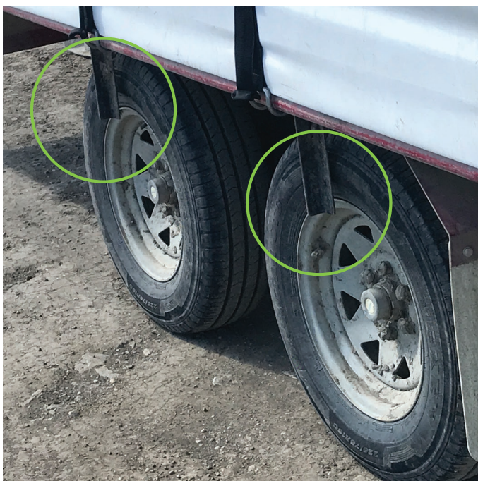
Figure 3.5: Examples of wheel scraper devices on vehicle wheels, to aid removal of soil.
