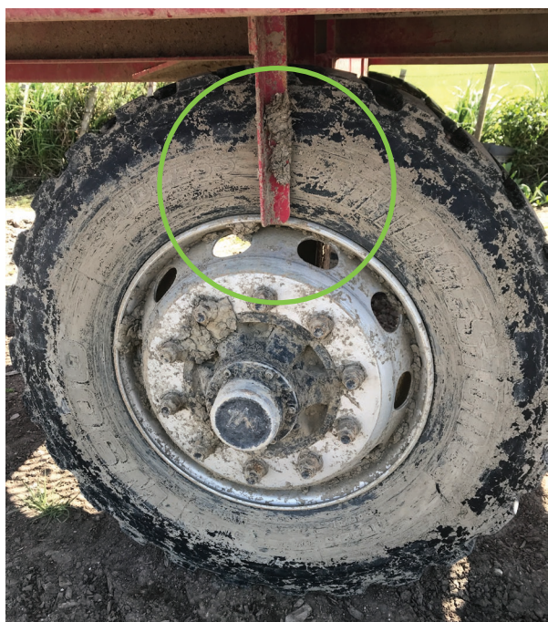
Figure 3.5: Examples of wheel scraper devices on vehicle wheels, to aid removal of soil.
